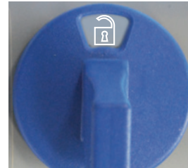
Hand control and/or nurse hand control unlocked
