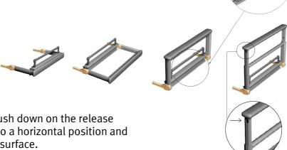
To store the assist rail, push down on the release bar, lower the assist rail to a horizontal position and slide it beneath the lying surface.
