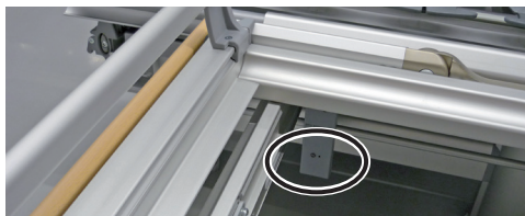
Cross end stop between upper and lower leg section.
