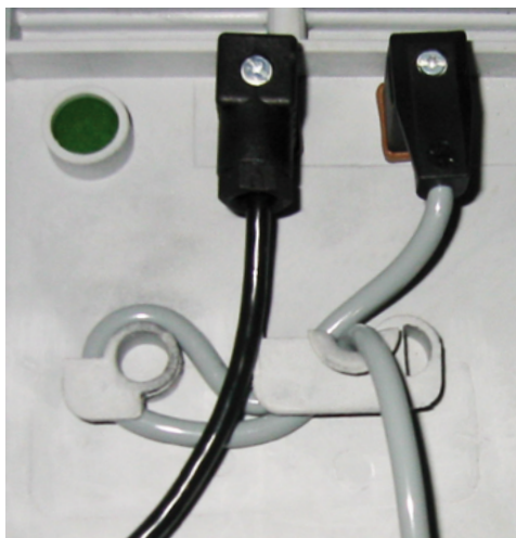
Routing the hand control cable
